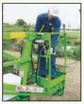
Integral harness point on platform for operator safety when working.
